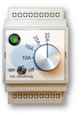
Picture 13: EVSE WB in custom box with 4 position current switch
